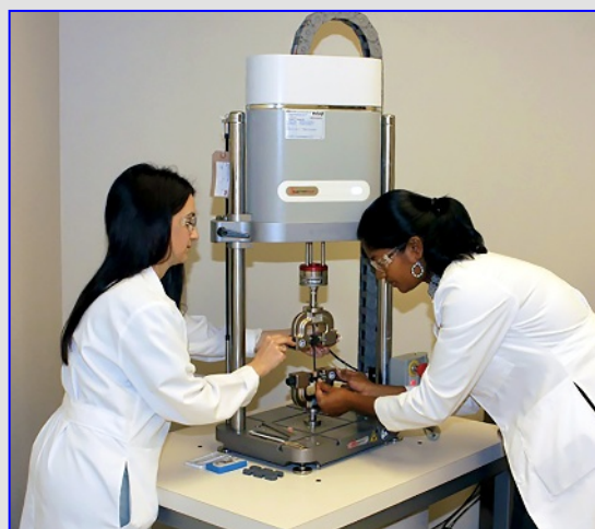
Dr. Melineh Dereghishian, a second year resident, assisting Dr. Prashanti Bollu with stabilizing a sample on the Instron E1000.
